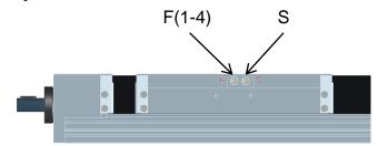
Lubrication of spindle drive **(S)**. Lubrication of guiding carriages 1 through 4 **(F)**.
